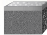
Efflorescence emerged from pores within a magnified area of a concrete paver. The calcium has been carried to the surface by water.
